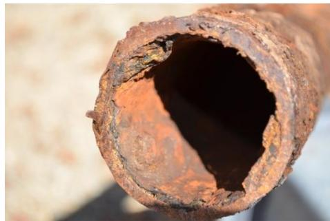
The above picture illustrates an interior view of a galvanized pipe with mineral deposits.
