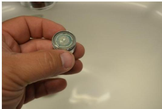
The above picture illustrates an aerator blocked with mineral deposits.
